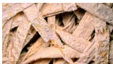
Figure 11. Microscope picture of a 2.0 mm fiber WWCB (Made by Veronica Caprai)
