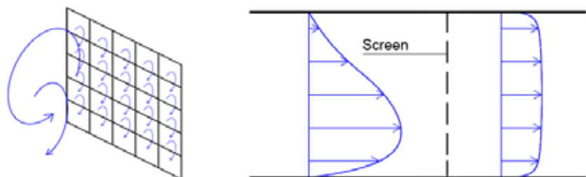
Figure 3. Principle of homogenizing the flow through a screen (a) and increased amount of uniformity of the wind flow due to application of screen (b)
